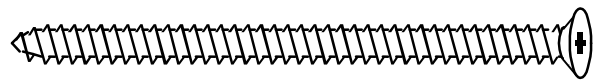
#12 X 2" (min.) SHEET METAL SCREW INTO JAMB (FURNISHED BY TIGER DOOR FOR BUTT HINGES, FURNISHED BY HINGE MANUFACTURER FOR CONTINUOUS HINGE)
