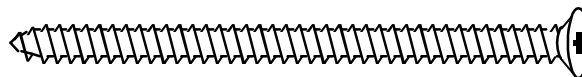
#12 x 3" SS SHEET METAL SCREW INTO DOOR (FURNISHED BY TD WITH DOOR)
