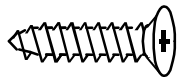
#12 x 3/4" (min.) Sheet Metal Screw into Jamb (Furnished by Tiger Door for Butt hinges, furnished by hinge manufacturer for continuous hinge)
